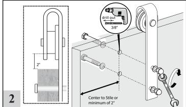
**INSTALL HANGERS** (See back for 2000, 5000, & 6000 Series Drawings) Position hangers on front center of stile (min. 2" from edge of door, equal on each side). Cut a piece of cardboard 2" high and place between the inner groove of the wheel and the top of the door to correctly position the height of the hangers. For 1000, 2000, & 5000 Series, mark holes & pre-drill 3/8" holes. Secure hangers. For 6000 Series, mark holes & secure hanger using screwdriver (do not drill.)
